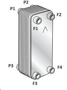
Ports F1/F2/F3/F4 are on the front of the BPHE. Ports P1/P2/P3/P4 are on the back. Note the order in which they appear.
