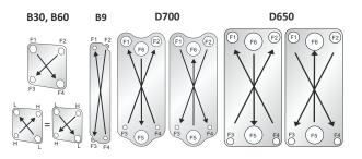
The B9, B30, B60, D650 and D700 have a cross-flow configuration, instead of the parallel flow normally found in BPHEs. In the B9, B30 and B60, ports F1-F4 are equivalent to the outer circuit, and ports F2-F3 to the inner circuit. For the D650 and D700, ports F5-F6 are the outer circuit and ports F1-F4 and F2-F3 are the inner circuits.
