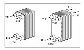
Danfoss 2 pass heat exchangers are made with 6 connections, as they are primarily used to heat tap water.
