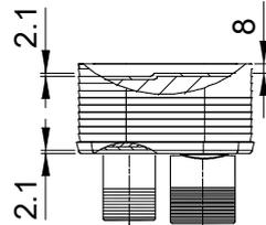
Frameplate is depressed 2.1 mm at connections S3 and S4 if holed.
