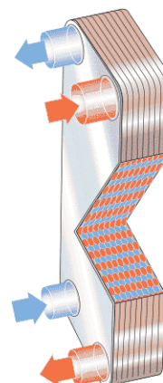
Flow principle of a brazed plate heat exchanger
