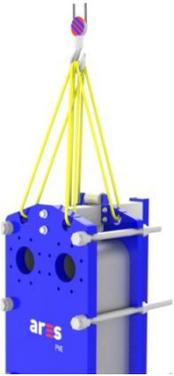
Please use lifting lugs when lifting and/or carrying the plate heat exchanger (A4,A6,A8, A12 and AWG models). Do not use any other part such as; bolts, carrying bar etc. to avoid any damage. Make sure the that the lines are equal and do not create imbalance when lifting the unit to prevent any injury.
